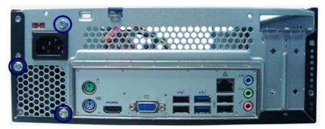
4. Pull the the power supply module toward the front.
